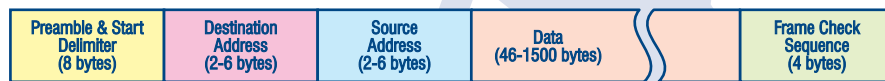
Fig.4: The basic format used in Ethernet data packets or 'frames'. Note the destination and source address fields, used in directing each packet around a network.
